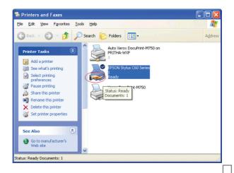
For a computer to access a Network Printer, the device driver or software for that printer must be installed and pointed to the proper location of the printer. This is done similarly to the way you installed the printer on the computer it is connected to.
